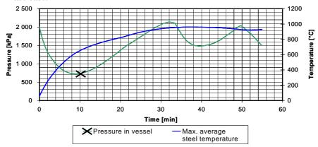
The figure above illustrates the pressure history for the demonstration case. That means no insulation and unit absorption coefficient.
